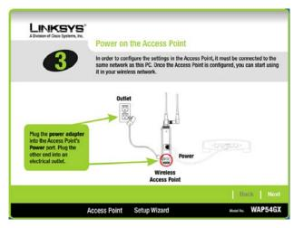
Figure 5-4: Power on the Access Point Screen
